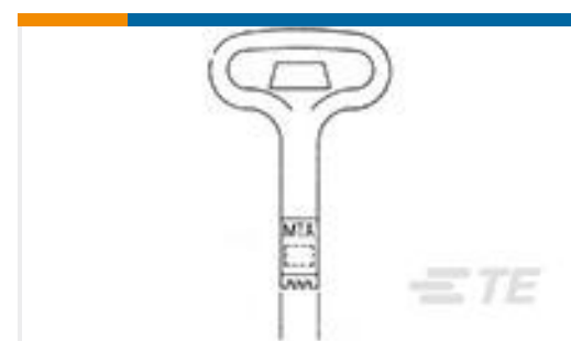
TE Part # 59804-1 MAINTENANCE TOOL
